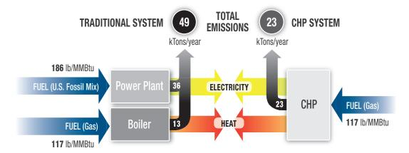
Example of the  ${\rm CO_2}$  savings potential of CHP based on a 5 MW gas turbine CHP system with 75% overall efficiency operating at 8,500 hours per year providing steam and power on-site compared to separate heat and power comprised of an 80% efficient on-site natural gas boiler and average fossil based electricity generation with 7% T&D losses.
