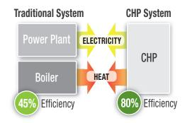
but it has quietly been providing highly efficient electricity and process heat to some of the most vital industries, largest employers, urban centers, and campuses in the United States. While the traditional method of separately producing usable heat and power has a typical combined efficiency of 45 percent, CHP systems can operate at efficiency levels as high as 80 percent.
